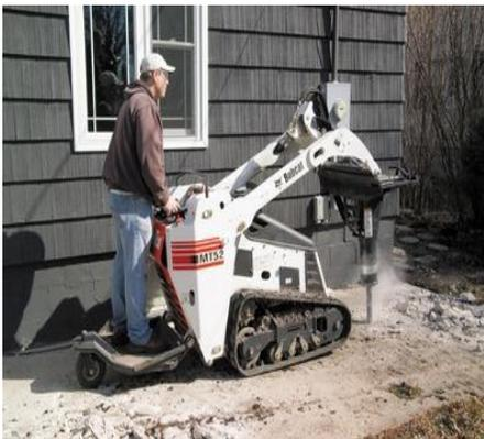
The 150 lb. is designed to be installed on the front of our walk behind track type skid steer. These walk behind loaders have the ability to work very tight areas that a full size loader could not go. In addition the walk behind offers greater production and less fatigue on the operator. Typically used on slabs up to 8".
